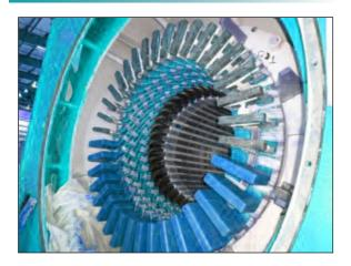
Stator Winding RTDs fit on the coil end of large motors and generators. Six sensors are recommended for each motors, two per phase. Locate sensors near the hottest point of the windings for best performance.
